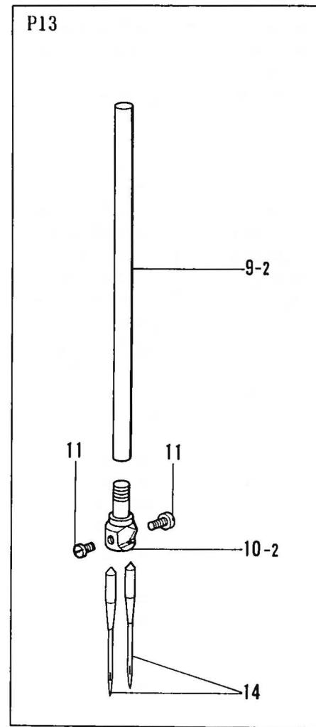
C. 針棒関係/Needle bar mechanism/Nadelstangenvorrichtung/
