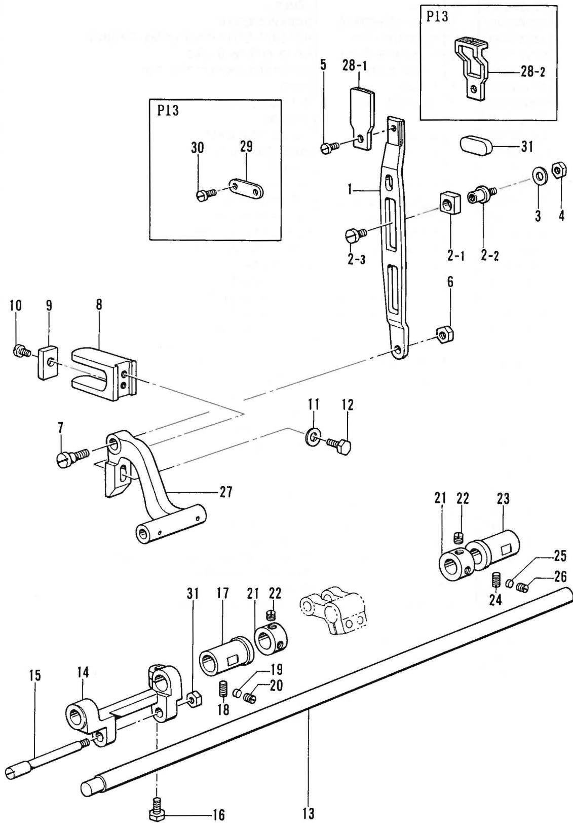
F. 上軸関係 /Upper shaft mechanism/Obere Welle/
