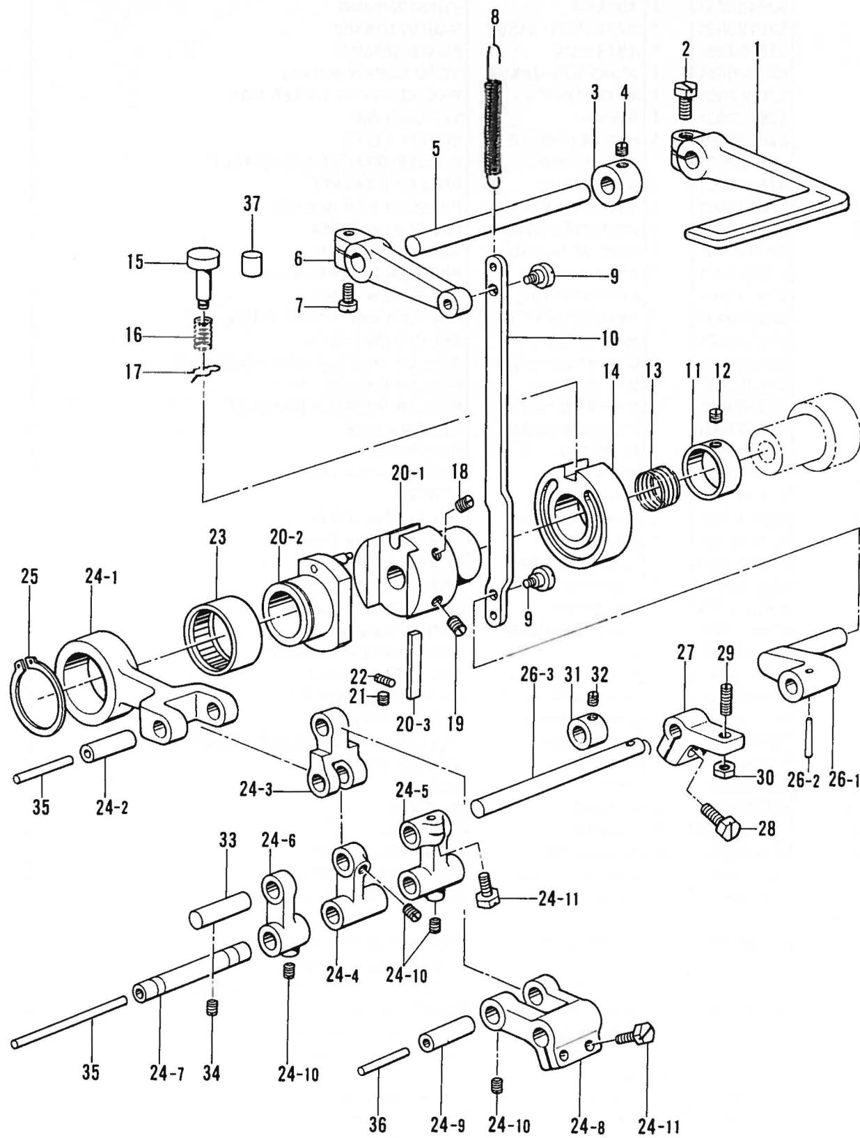
E. 送り関係 /Feed mechanism/Transportvorrichtung/
